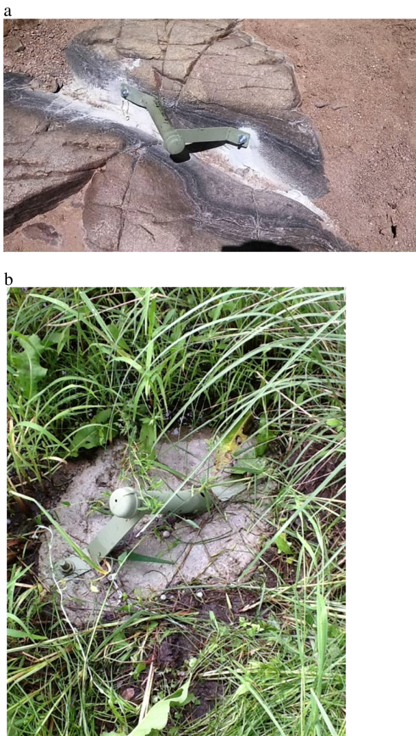
Figure 3. Photographs of steel holster constructed to house the leveloggers at (a) untreated watershed and (b) treated watershed. This figure is available in colour online at wileyonlinelibrary.com/journal/rra
